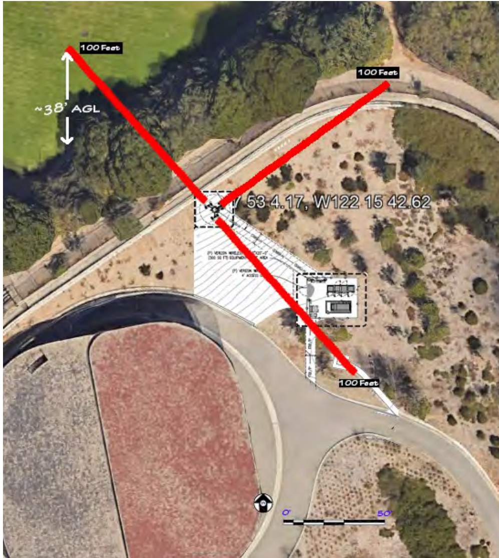
Figure 8: Approximate (i) location of monopine, and (ii) azimuth orientations for all three sectors (Source: Google Earth Pro, Applicant's Plans; annotations by Dr. Kramer).
