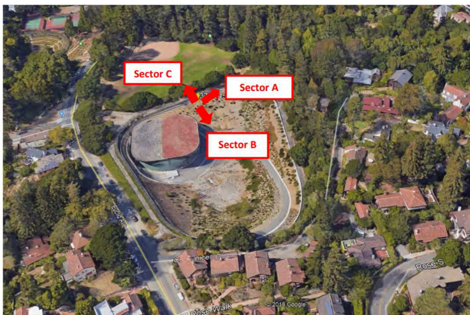
Figure 8: Approximate (i) location of monopine, and (ii) azimuth orientations for all three sectors (Source: Google Maps; Annotated by Dr. Kramer).
